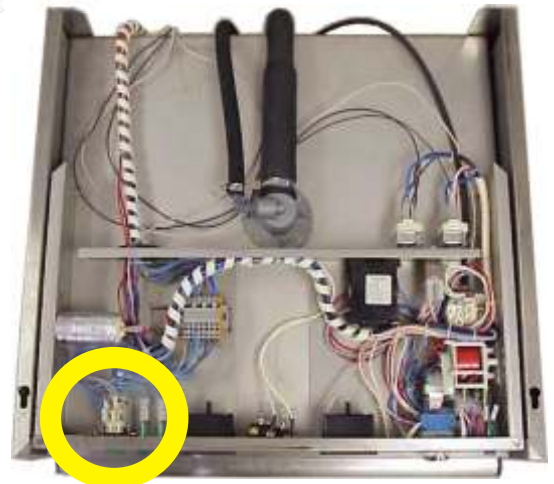
Power Switch Location
